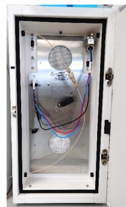
This photos shows the location of the union (instead of flow cell during flush) in the detector oven.
